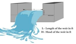
The height of spillway is usually not kept more than 0.75m. Therefore for the selected catchment length of the spillway
