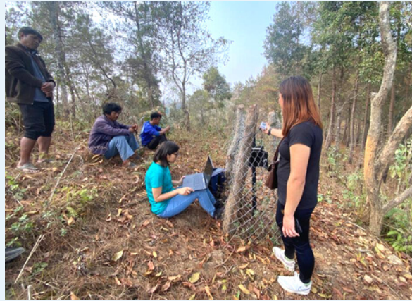
Extraction of data from soil moisture sensor installed at Khlieh Umtrew.
